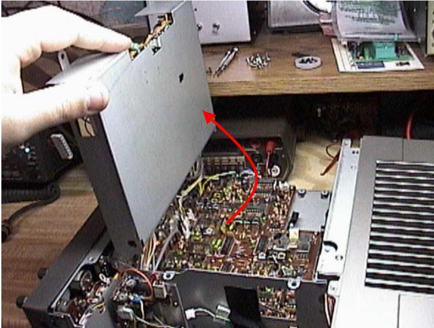
The IF board will swivel up on a hinge exposing the PLL Board. It may be necessary to unplug a few cables on the IF board to get it to lift up.
