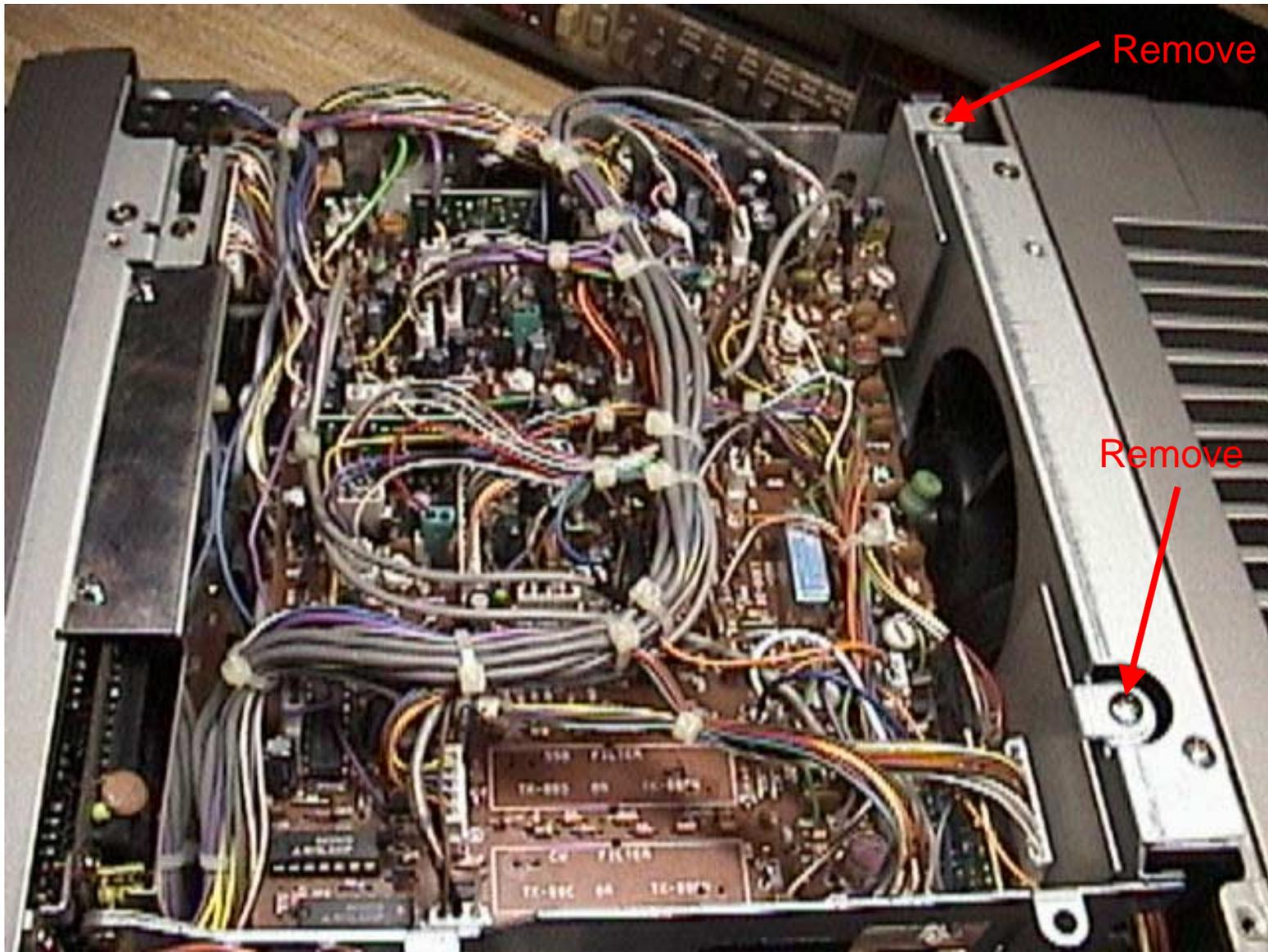
This is the TS-440S with no top cover. You can see the IF Board. Remove the two screws to expose the PLL board underneath.
