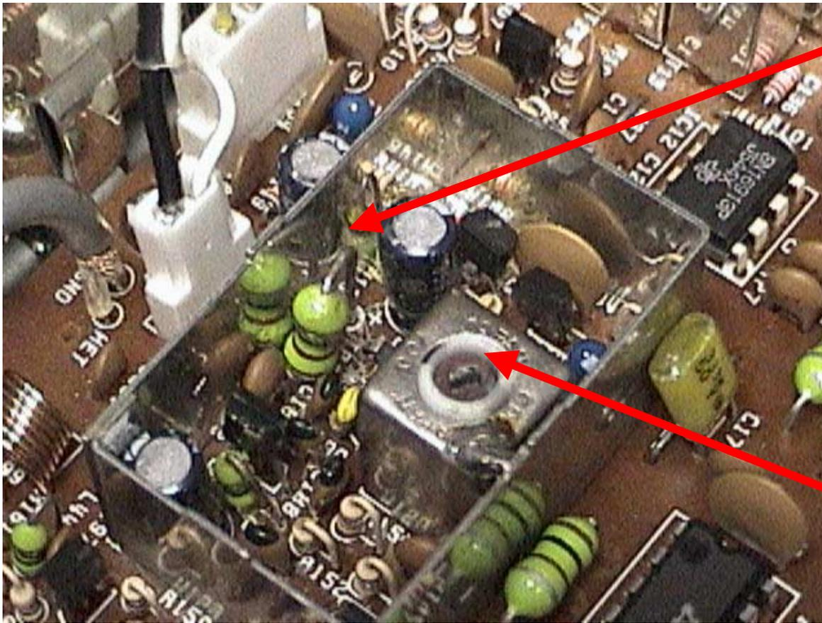
TP11. Exposed end of Inductor. This is where you want to take a voltage reading from. Connect the red lead here, and the black lead to any point on the chassis (ground).
