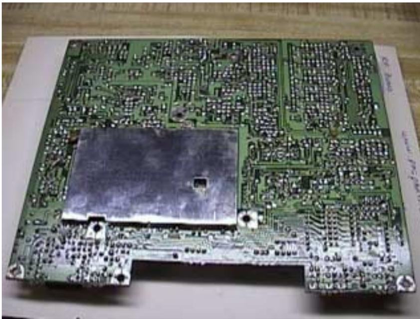
RF board removed (solder side) with shield.
